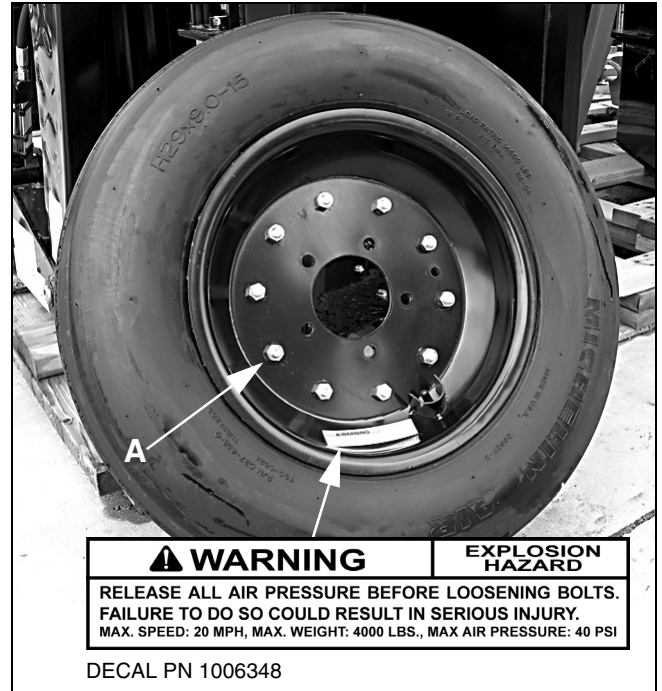
Figure 10. Split Rim Tire Servicing
